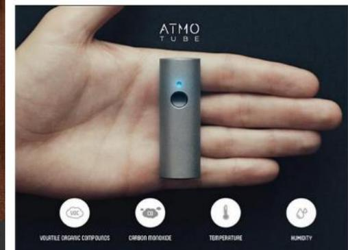
The Atmotube wearable air pollution sensor sends local air quality data to a user's smartphone in real time.
